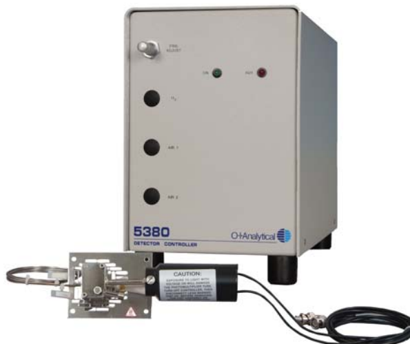
Figure 1. Pulsed Flame Photometric Detector (PFPD) used for detection and quantitation of thiophene in benzene by ASTM methods D4735 and D7011.
